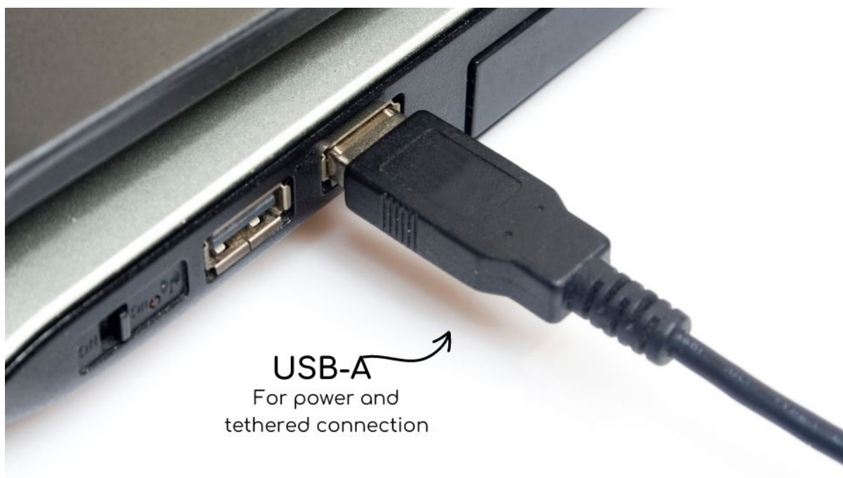
Fig. 2.5: USB Connection to the PC/Laptop
