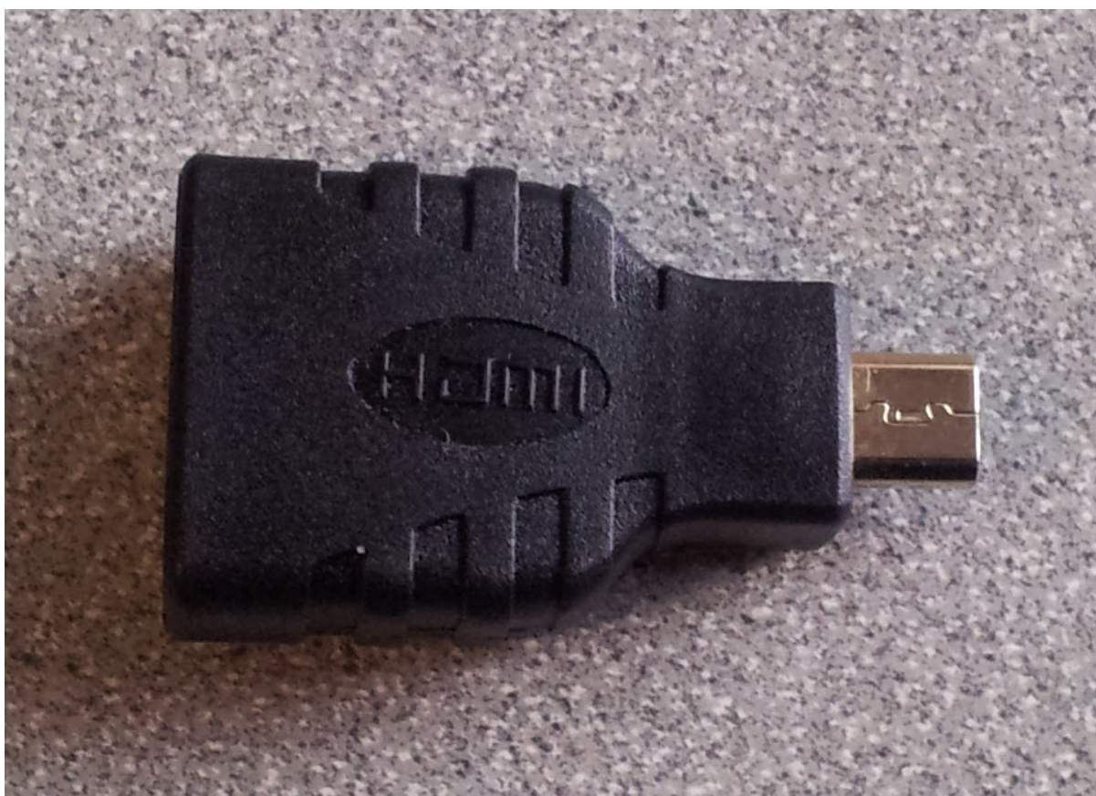
Fig. 5.1: Female HDMI-to-male microHDMI adapter
