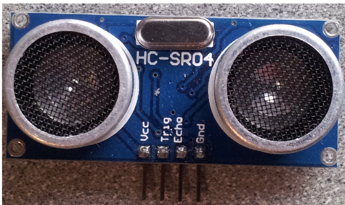
Fig. 2.12: HC-SR04 Ultrasonic range sensor
