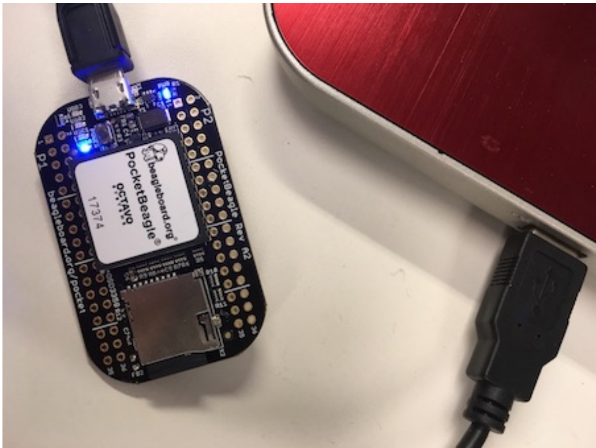
Fig. 3.12: Insert the USB connector into PC
